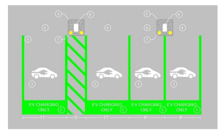
Note: Typical detail. An additional access isle has been added to the design for ADA compliance in this particular location. See page 2 for details.
